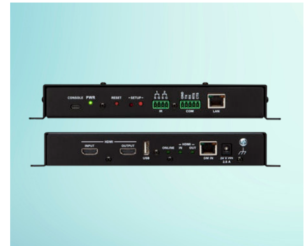
AM-300 AirMedia Presentation System with AirMedia 2.0, DM® in, and HDMI in and out
